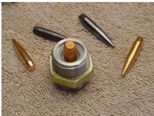
Figure 9 - Meplat projectile holder with projectile inserted.
