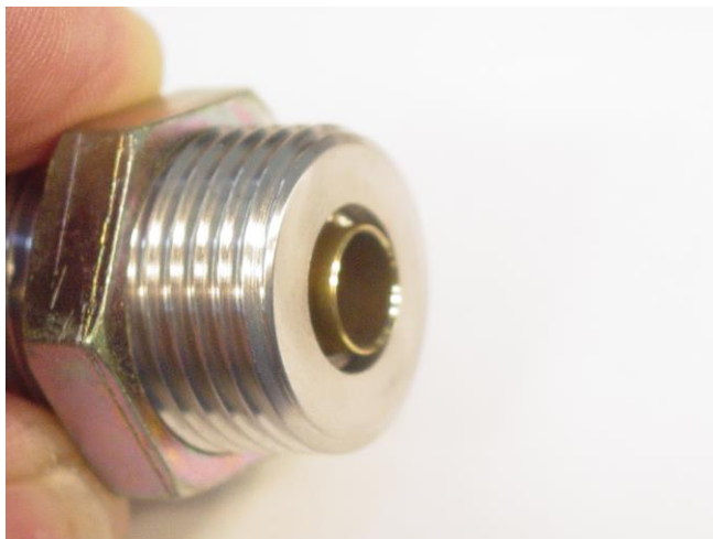
Figure 4 - Case inserted into the case holder, but not depressed against the compression spring,
