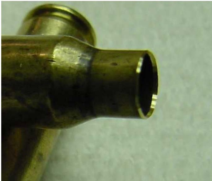
Figure 12 - Freshly trimmed case mouth showing proper inside and outside chamfers.
