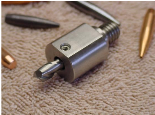
Figure 8 - Meplat cutter head with carbide end mill.
