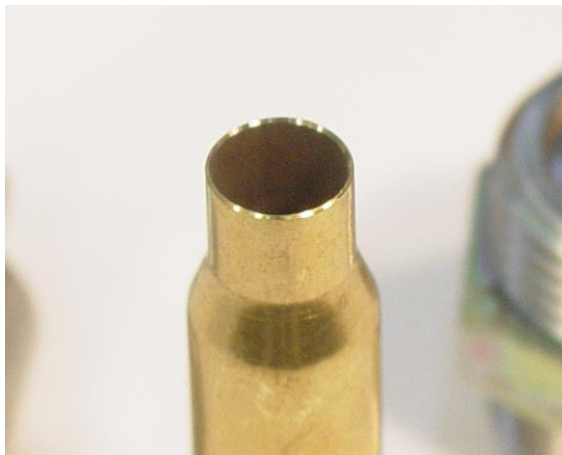
Figure 2 - A properly trimmed case has a chamfer that is even and smooth around the entire case mouth, both inside and outside.
