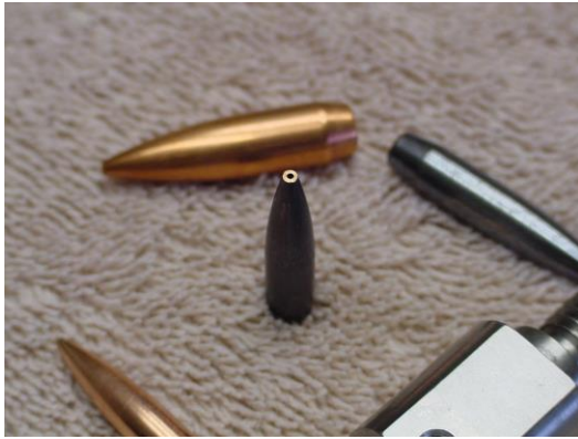
Figure 10 - Meplat trimmed projectile, showing uniform trimmed surface.
