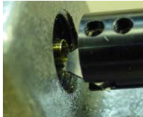
Figure 8 - Case mouth aligned and securing cutting blade for tightening of the set screw.
