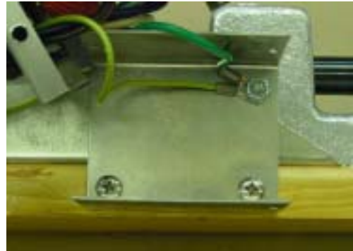
Figure 4 - Motor switch box mounted on edge of base.
