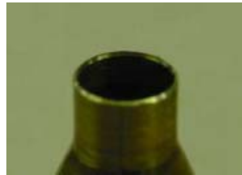
Figure 9 - Case mouth showing proper adjustment of the cutting blades with even chamfers on inside and outside surfaces.
