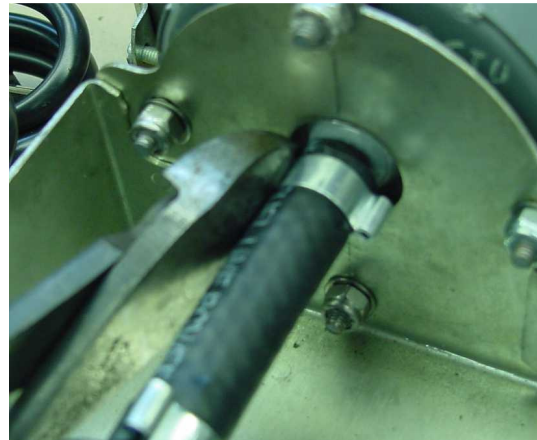
Figure 6 - Crimping the band clamps around the drive hose with side cutting pliers.
