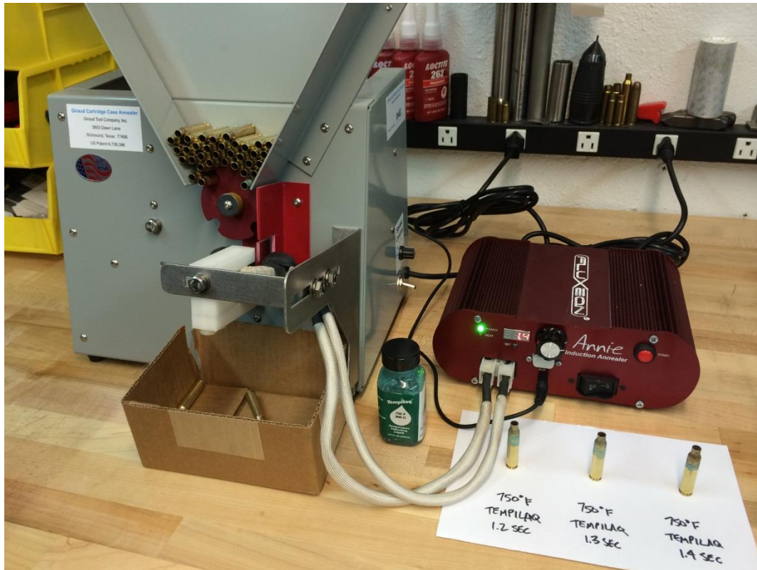
Figure 4 - Annie Induction power supply connected to the annealer showing the display, phono cord, and ferrite core connections.
